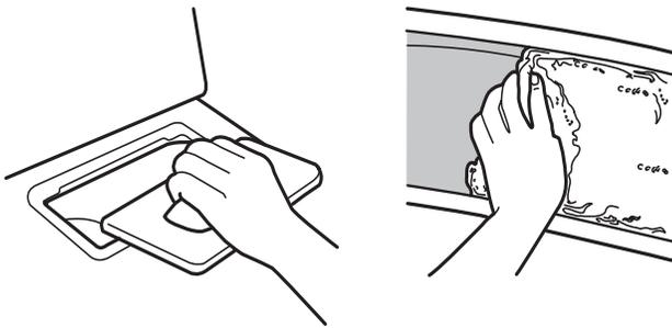
Clean the lint screen before each load. Pull the lint screen out of its holder. Roll lint off the screen with your fingers. Do not rinse or wash screen to remove lint. Push the lint screen firmly back into place.
